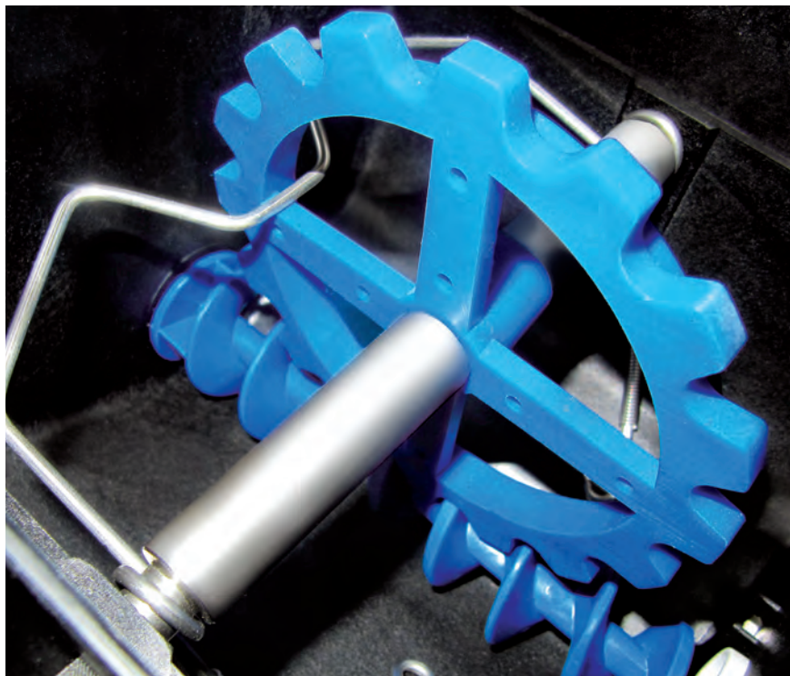
MicroPowder dosing with globoid screw and stainless steel agitator
