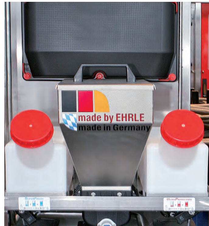
Chemical dosing level with MicroPowder dosing and liquid chemical dosing
